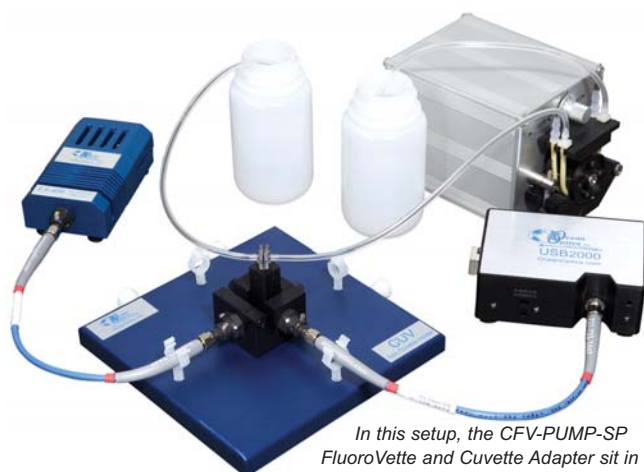
Detection of fluorescein in the nanomolar range (nM) is typical with FluoroVettes. These spectra were made with a CFV-PIP-SP, USB2000-FLG Spectrometer, LS-450 Blue LED, CUV-ALL-UV Cuvette Holder, 1000 \mu\text{m} illumination fiber and 600 \mu\text{m} read fiber. The integration time was 1000 msec; a longer integration time provides even lower detection limits.
