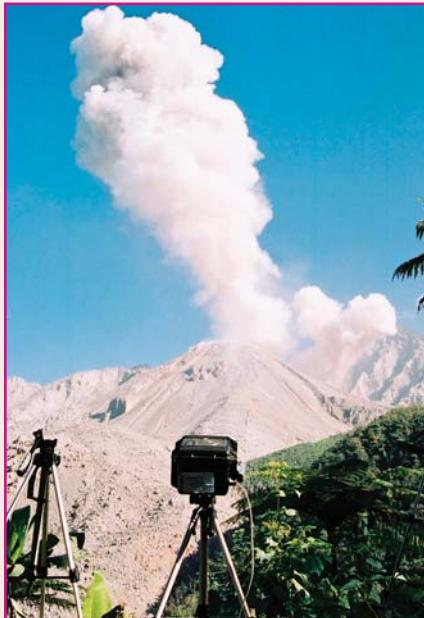
At the Montserrat Volcano Observatory ([www.mvo.ms](http://www.mvo.ms)) sampling sites, spectra are collected every 4-6 seconds and transmitted to researchers at the observatory via modem; one complete scan of the plume takes 4-6 minutes. Depending on wind direction, data from two of the three spectrometers is used to calculate plume height, by comparing the angles at which peaks in the  $\text{SO}_2$  plume are measured.
